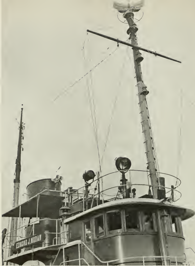
LEFT: RADAR ANTENNA OF THE "MORAN" IS LOCATED AT PEAK OF FOREMAST.
