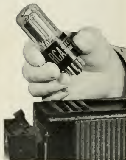
THIS TINY RCA PHOTOTUBE TRANSFORMS LIGHT VARIATIONS OF ULTRAFAX MESSAGES INTO RADIO SIGNALS.
