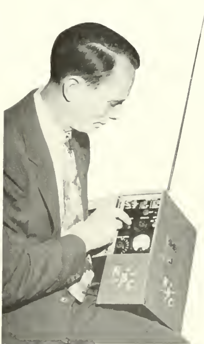
J. L. HATHAWAY HOLDS THE LATEST STREAMLINED MODEL OF THE PACK TRANSMITTER. BATTERIES TO OPERATE THE UNIT FOR 6 HOURS ARE INSIDE THE CABINET.
